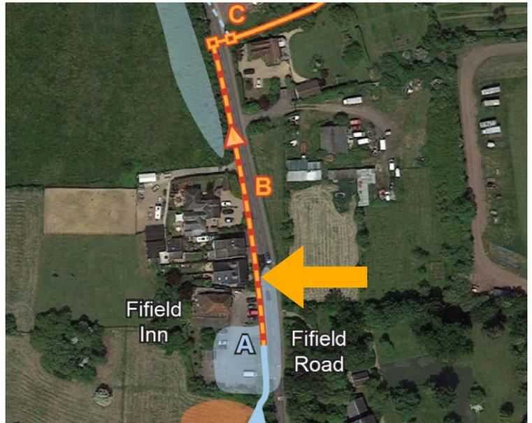
**Wet Spot 7B** from south of the Fifield Inn northwards to the same chamber at Garden Cottage has been dysfunctional for a very long time. The problem starts at the pipe under the entrance to the pipe car park which simply has inadequate capacity and backs up eventually into the car park as seen many times and shown below.
